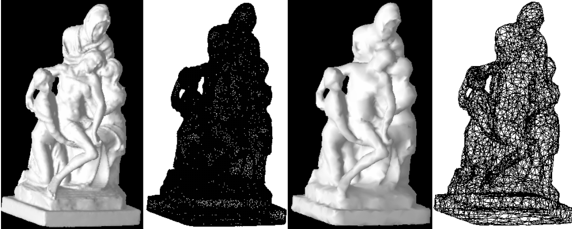
Figure 1. In computer graphics, a solid object (leftmost image) is often represented as a dense mesh of triangles (second image from left.) To facilitate interactive display performance, objects are often simplified (third image from left), to reduce the number of triangles (rightmost image), while attempting to preserve the appearance of the object.
